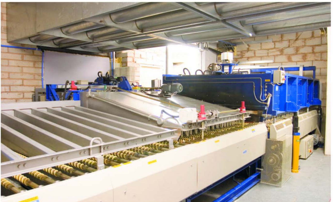
The EFCO glass-tempering system with a 3000mm x 1500mm load area
